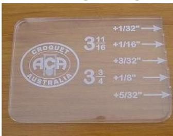
The Wedge Gauge is an acrylic gauge weighing approximately 50 grams, which is much lighter than a brass gauge, and can be used when setting hoops to all of the specifications set down in the TRegs for both level play and handicap play at all levels of GC competition.
