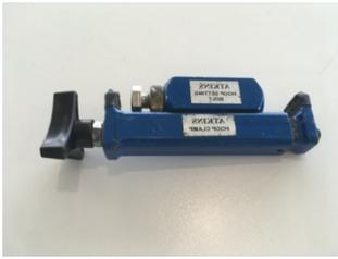
The Atkins Setting Bolt & Clamp are invaluable when setting Quadway (and other) hoops for WCF requirements, i.e. all hoops on a court set to the largest ball plus 1/32".
