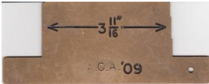
The **ACA '09** gauge is a brass gauge with three measurements,  $3 \frac{11}{16}$  inches,  $3 \frac{23}{32}$  inches and  $3 \frac{21}{32}$  inches, which allows for checking that the distance between hoop uprights is within the allowable range for level play events.
