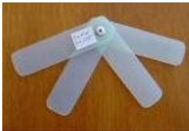
Hoops width settings may sometimes be measured at half ball height above the court surface using the ball with the largest diameter plus  $\frac{1}{64}$  inch,  $\frac{1}{32}$  inch or  $\frac{1}{16}$  inch. Therefore, the hoop setters, and official responsible for checking the hoops, needs to have access to a set of feeler gauges for all three measurements. This technique is more time consuming than other methods but it is commonly used in WCF
