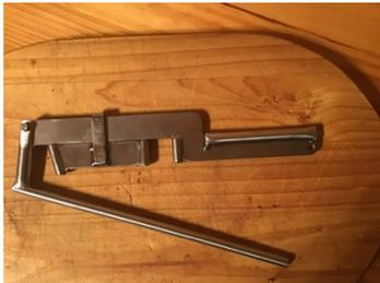
The clamp pictured was designed and manufactured by Ian Bassett and is designed to hold the hoop at  $3\frac{11}{16}$  whilst setting it into the ground. These clamps are found at several clubs within Victoria.
