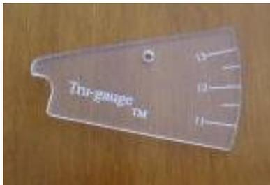
The Tru-gauge™ is a rigid plastic gauge with an arc shaped edge graduated in  $\frac{1}{32}$  inch steps from  $3 \frac{11}{16}$  inches to  $3 \frac{13}{16}$  inches.
